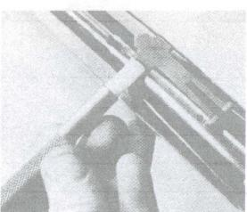
Riex the rear sight very slightly upward, and take out the sight elevator. Drifting out the rear sight toward the right will release the barrel collar cover for removal upward, giving access to the barrel collar.
