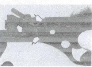
The feed system is retained by three cross-pins.
