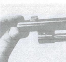
Drifting out the small, short cross-pin in the magazine tube hanger near the muzzle will release the outer magazine tube for removal toward the front. This will allow the fore-end to be taken off downward. After removal of the fore-end, the nylon fore-end mount is easily slid out of its dovetail toward either side.
